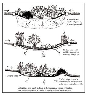
**Installation:** Rain gardens can vary in size, but are most effective when built to 20-30% of the drainage area. Rain gardens for single-family homes will typically range from 150 to 300 square feet, but even a smaller one will help reduce water pollution problems.
